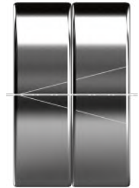
Outer raceway markings for paired bearings
